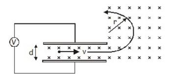
plates where only the magnetic field exists, it trajectory is circular with radius r = 0.250 m.
